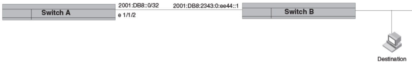
FIGURE 18 Example of a Static Route
